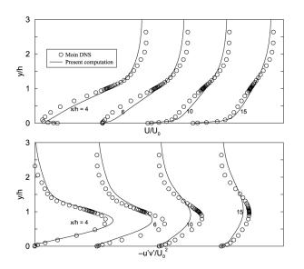
Figure 2. Backward facing step: velocity and Reynolds stress profiles
