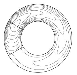
**Figure 4.** Buoyancy driven loop: temperature field
